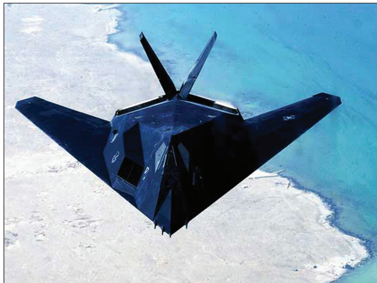
Lockheed 117 Nighthawk Stealth Fighter – this tailless aircraft called a flying wing uses elevons as control surfaces for pitch and roll control. The elevons are not part of the main wing but instead are a separate tail surface.
